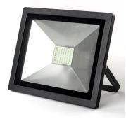
The Tatton is a Class I product and must be earthed. Available with or with out PIR Detector with black body. PIR detection distance: 8m max Mounting height: 2-4m. Time delay 10 sec. to 10 min. Adjustable sensitivity and day/night operation. PIR versions have a fourth black wire providing manual over-ride, connection diagram below.
